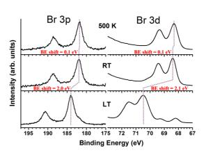
Figure 3. Br 3p and Br 3d core level spectra for dBB on Cu(110) deposited at different temperatures using an incident photon energy of 390 eV: 1 monolayer (ML) deposited at LT, RT, and annealed at 500 K.
