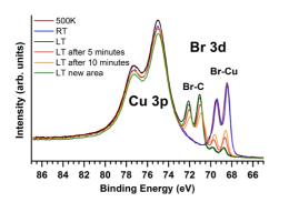
Figure 2. Br 3d and Cu 3p core level spectra for dBB on Cu(110) deposited at different temperatures using an incident photon energy of 390 eV: 1 monolayer (ML) deposited at low temperature (LT), investigated as a function of the exposure time to the synchrotron radiation and of the position of the beam on the sample, 1 ML at RT and annealed at 500 K.
