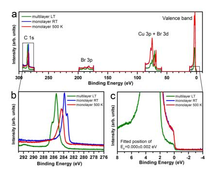
Figure 1. XPS spectra for 1,4-dibromobenzene (dBB) on Cu(110) deposited at different temperatures using an incident photon energy of 390 eV. Fermi level of each XPS spectrum was aligned to BE = 0 eV. The BE shifts in the C 1s and Br 3d peaks are clearly not related to calibration problems as demonstrated by the magnified regions of C 1s (b) and Fermi level (c) of the wide spectra (a).
